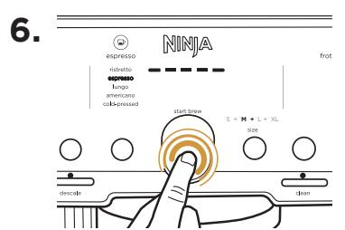
Press **START BREW**. The machine will beep to signal the brew has started. The progress bar will illuminate, indicating the status of the brew.
