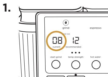
Check to see if the current grind setting matches the recommended setting.
