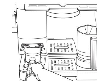
Release the tamper lever and remove the portafilter from the grinding cradle.
