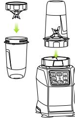
2. Fill the cup with desired contents and screw on blade assembly clockwise until you have a tight seal.
