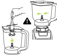
2. Holding the stacked blade assembly by the top of the shaft, insert it into the pitcher.
