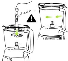
2. Holding the desired blade assembly by the top of the shaft, insert it into the bowl.
